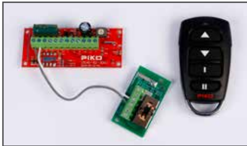
35040 R/C Sender und Empfänger 86,00 €* 35040 R/C Loco Receiver, 3A, w/Pocket Remote
